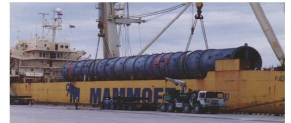
Delivery of a 165-ton column, 56 meter long, 6.4 meter diameter
