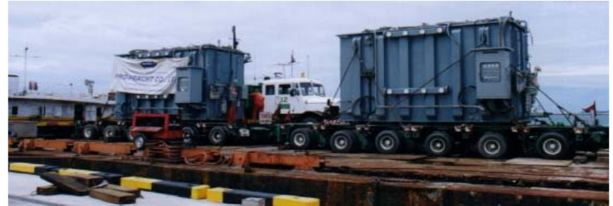
Loading two 98-ton Transformers on a flat top barge at Laem Chabang Port
