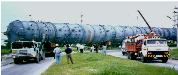
Delivery of a 465-ton column, 84.5 meters long, 6.8 meters diameter
