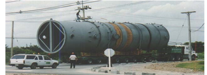
Delivery of a 215-ton column on multi-axle modular hydraulic trailer
