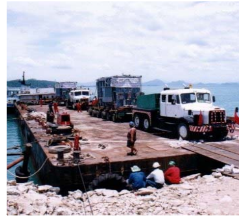
After grounding and securing the barge, the Transformers can safely be rolled off.
